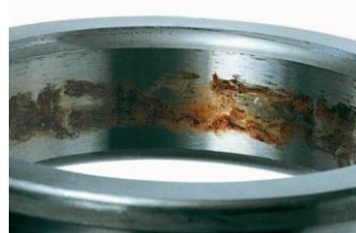
Typical damage of corrosion
