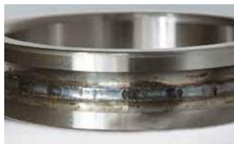
Typical damage of wear
